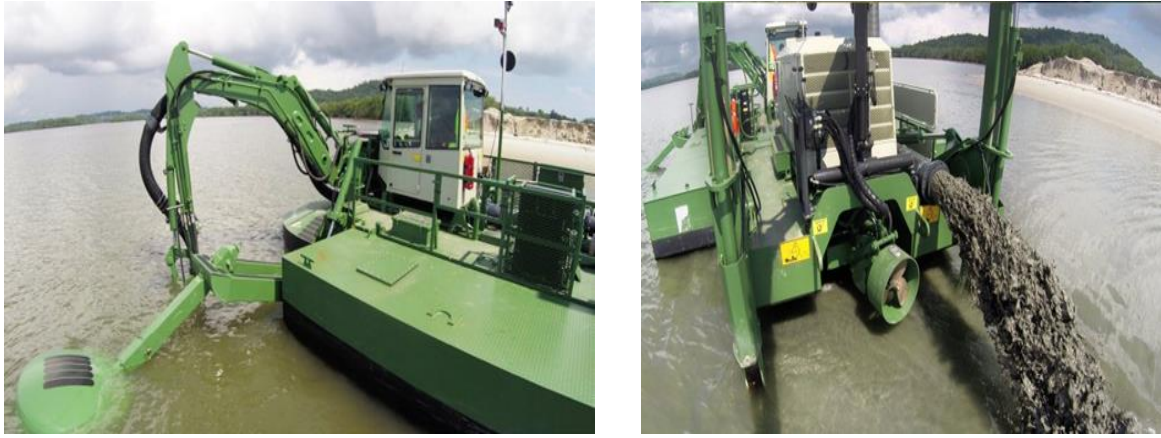
Figure 3.4. Watermaster Amphibia Dredger in operation.
