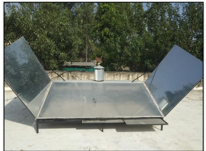
Fig. 2. Developed solar conduction dryer.
