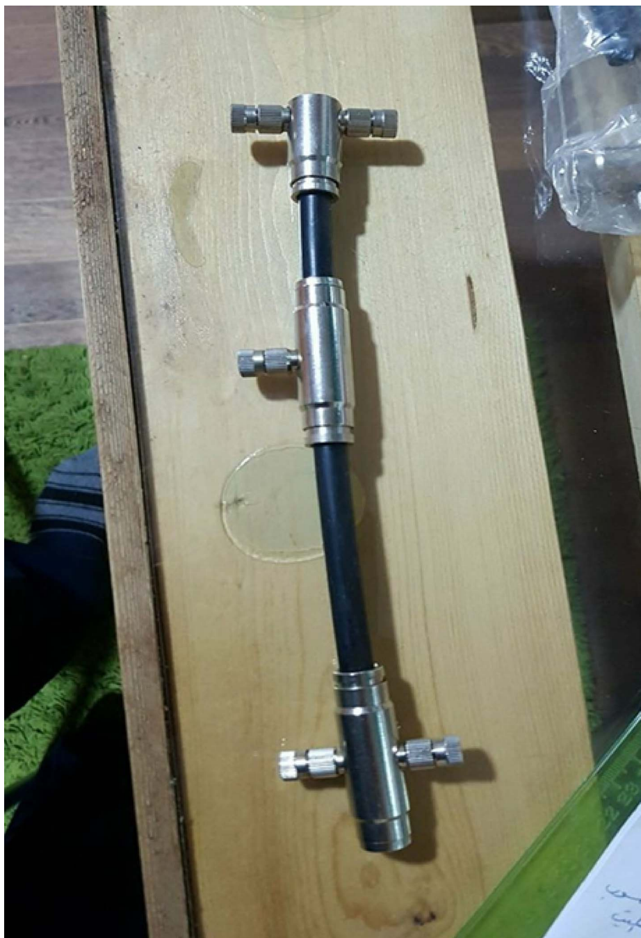
Figure 3. A sample of the nozzle of the fogging system chosen in 'Khodra'-Jordan.
