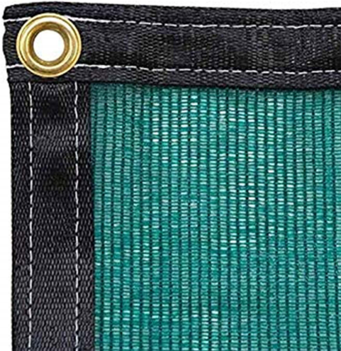
Figure 2. Green knitted 50% shading cloth used in 'Khodra'-Jordan.
