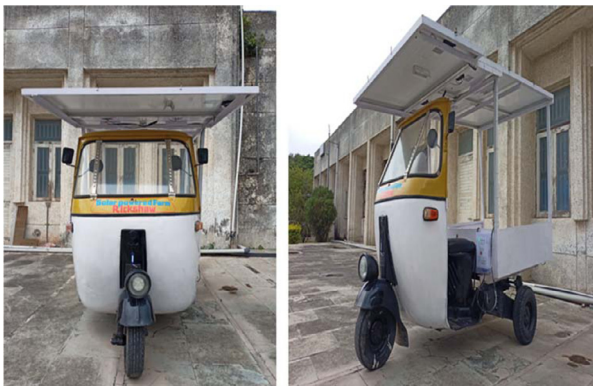
Fig. 6. Different views of developed solar powered farm rickshaw.
