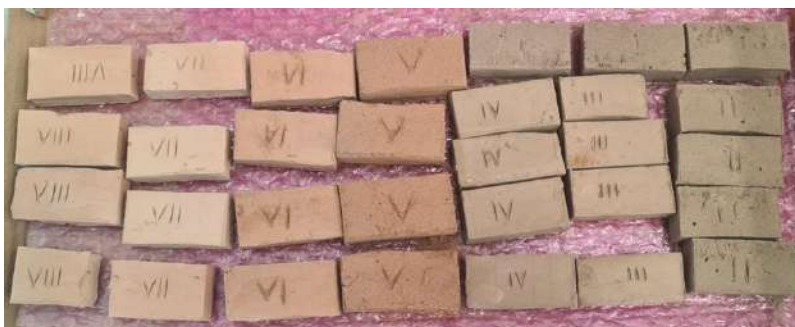
Figure 2: The ready sample product (bricks), made using the samples of the Ruslovoe reservoir sediment
