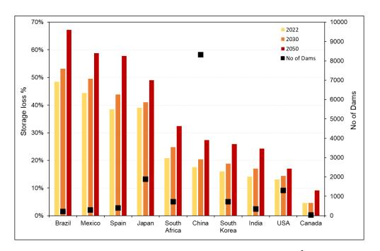
Figure 6. Storage loss estimates for the dams of capacity under one million m<sup>3</sup>.
