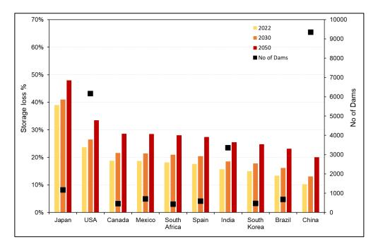
Figure 7. Storage loss estimates for the dams of capacity over one million m<sup>3</sup>.
